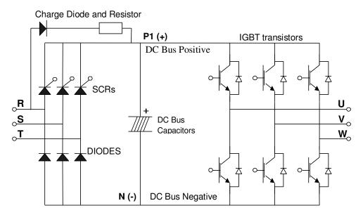
Note: The 50-700HP VFDs have half controlled rectifier bridge with SCRs (silicon controlled rectifier). The SCR cannot be checked for conducting state with multimeter. The reading from R to P1 terminals will represent charge diode and resistor circuit. Terminals S and T to P1 will show closed state in direct and reverse test if SCRs are not shorted.
