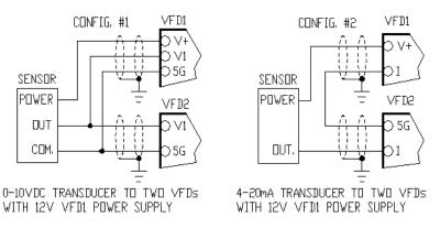
power supply. **Configuration #1** Two or more VFDs connected to one 0-10VDC transducer fed by VFD1 12VDC internal power supply. **Configuration #2** Two VFDs connected to one 4-20mA transducer fed by VFD1 12VDC power supply. If VFD1 is not powered, 4-20mA loop is not powered and VFD2 cannot operate properly on PID control without feedback signal. If VFD2 is not
