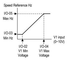
V1S mode. VFD frequency is controlled by bipolar  $\pm 10$ VDC analog input signal from PLC, potentiometer or other control device. The polarity of the signal corresponding to analog common 5G (up to 40HP) or CM (50HP and larger) determines Forward or Reverse direction and the absolute value of the signal changes the speed reference. Use shielded cable because voltage input is sensitive to any electrical noise. The input range is adjustable in I/O group parameters up to  $\pm 12$ VDC.
