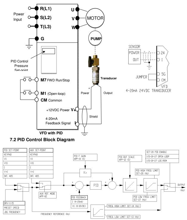
The picture above shows a PID block diagram with most of the required PID operation parameters. The PID output (Target) and VFD output frequency (Out) can be viewed on parameter DRV-25 screen.
