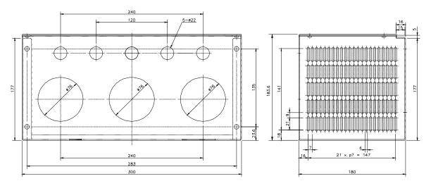
Conduit box for 100~125HP VFD
