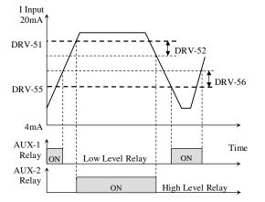
Note: If better accuracy required for analog level monitoring feature, use parameters MAK-37 and MAK-38 for analog mA signal calibration
