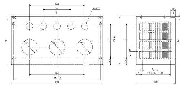
Conduit box for 050~075HP VFD
