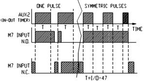
The timer set to ONE Pulse mode will generate one pulse for duration set in I/O-47 after input was activated momentarily or continuously. The timer set to Symmetric Pulses mode will generate pulses with identical ON and OFF duration set in I/O-47 when input is activated. **I/O-47** is a In-Out timer time setting in seconds. The default setting is 30 seconds and can be changed in 0-6000 range.
