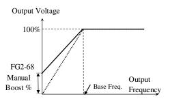
for Forward Boost and FG2-69 for Reverse Boost. The Torque Boost value is a percentage of SET-08 Motor Voltage.
