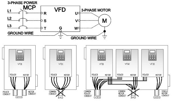
VFD can malfunction or be damaged if motor and power wires are in the same conduit or motor wires from two or more VFDs are in the same conduit!
