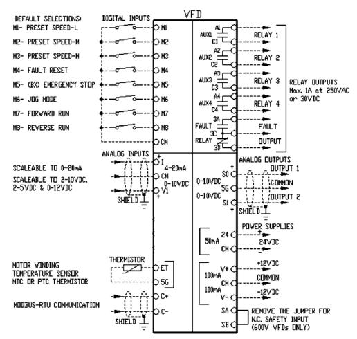
Note: Use terminal CM for analog inputs and ±12VDC power supply common.
