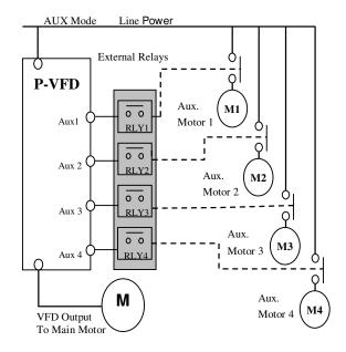
**Main-** the alternation mode is enabled and VFD will alternate auxiliary motors on the VFD output by run time timer.
