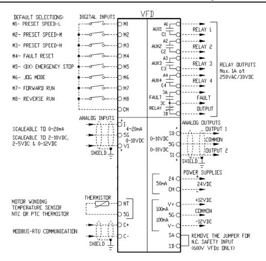
Basic types of analog inputs wiring with 5G common terminal
