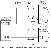
0-10VDC TRANSDUCER TO TWO VFDs WITH 24V VFD1 POWER SUPPLY
