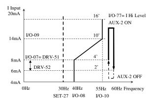
2<sup>nd</sup>. Set AUX relay for low level trigger and wire it to M5 Emergency Stop input. Set I/O-77 to I Lo Level, DRV-55 to 6mA and DRV-56 to 2mA. Wire AUX-2 relay contact between VFD M5 and CM terminals. When water level is above 2' AUX-2 relay contact is open and VFD runs. When water level drops below 2', AUX-2 relay closes its contact and VFD stops by BX fault. The VFD will start again when water level rises above 4' level and
