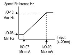
V1+I mode. VFD speed is controlled by both 0-10VDC and 4-20mA analog input signals from BMS, PLC, potentiometer or other control device. Both analog signals are compared with each other and the greatest value determines the VFD speed reference. The VFD speed reference can be switched between V1 and I inputs by digital input set to ANA\_CHG (Analog change). The input ranges are adjustable in I/O group parameters.
