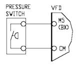
Install on the system piping properly sized pressure switch and wire its N.O. contact to VFD's CM and M5 (BX Emergency Stop) terminals. By default I/O-30 parameter is set to Yes (Automatic Reset for BX trip) and VFD will restart when cut-off pressure switch contact is open again. In case if only manual reset is acceptable, change I/O-30 setting to No. The wiring diagram shows pressure switch connection to VFD terminals.
