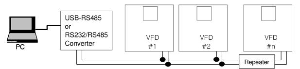
Note: The repeater is used for long-distance communication or high noise environment.
