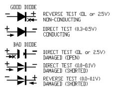
The VFD input and output power components are semiconductors and can be checked by multimeter with diode check mode ( $\bigstar$ ). When DC voltage positive is applied to the diode anode (triangle  $\blacktriangleright$ ) and negative to cathode (bar []), the diode is conducting.
