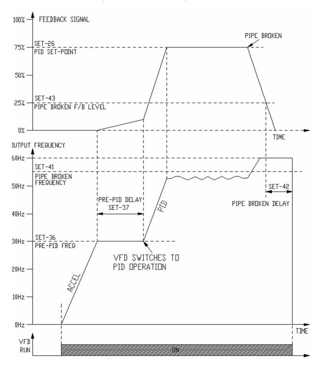
7.4 PID control with Pipe Broken function diagram.
