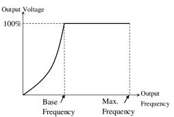
**User V/F** pattern is used for special applications with up to five different Volts/Frequency ratio step requirements. The User V/F curve can have one or two standard V/F segments and up to three custom V/F ratio segments. The parameters FG1-41~48 define Voltage and Frequency for each point on the User V/F curve.
