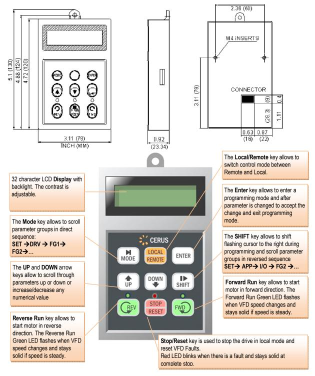
Note: 1. Both green LEDs may flash during normal operation when run sequence activates internal time delays or during Auto Tuning and Pre-Heat modes.
