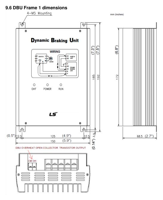
Note: Open collector transistor output is N.C. type. When DBU is not powered, OH output is open and will be closed when power is applied and DBU is not overheated. When DBU is powered and overheated, the OH output will be open.
