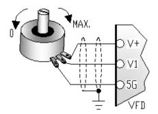
VFD speed control potentiometer wiring with VFD internal 12VDC power supply. The recommended potentiometer parameters: Resistance from  $1k\Omega$  to  $10k\Omega$  and Wattage 0.5W or higher. The multi-turn potentiometer provides more precise speed adjustment compare to a single-turn potentiometer. The internal power supply provides 12VDC and in order to have full range of speed control by potentiometer, change the I/O-04 parameter from 10VDC to 12VDC.
