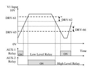
Note: If better accuracy required for analog level monitoring feature, use parameters MAK-35 and MAK-36 for analog voltage signal calibration.
