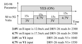
Note: For VFD's 50HP and above the I input test with S0 output does not work (it will read the maximum value 4095).
