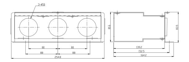
Conduit box for 030~040HP VFD
