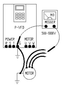
The windings insulation resistance should be in the Mega Ohm range.
