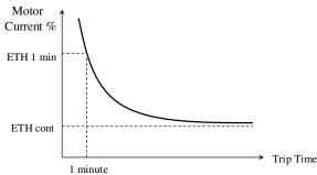
FG1-62 sets the service factor current (SFA) as a percentage of the motor FLA for continuous run. Note: For submersible pump application FG1-62 is set to 100% and SET-03 should be set to motor SFA not FLA.
