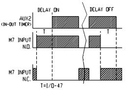
The following diagram shows timer operation in ONE Pulse and SYMM. Pulse modes with M7 as N.O. and N.C. contact and AUX2 relay set as a timer relay.
