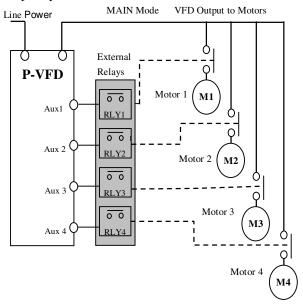
**APP-67-** the alternation run time timer setting is in hours. The VFD counts only run time and when it exceeds APP-67 and VFD output frequency is lower than APP-68 setting, VFD stops the motor, deactivates its relay, then closes next motor relay and starts again.
