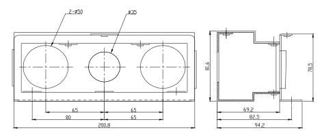
Conduit box for 020~025HP VFD
