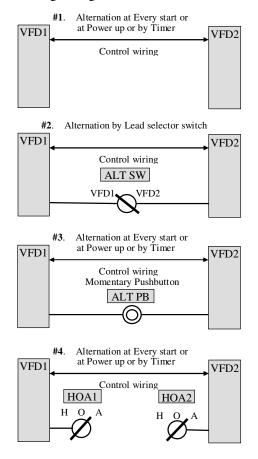
**The configuration #1** is for two VFDs with only control wiring between them. The alternation mode can be set to By Timer, At Power up or can be configured for alternation at Every start.
