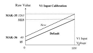
Note: Resetting VFD parameters to factory default settings in parameter FG2-93 with reset both analog inputs calibrations in MAK group.
