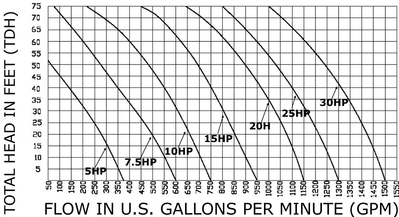
**PLOT YOUR POINT:** Follow the flow in U.S. gallons per minute required horizontally on the chart to your GPM flow required; then follow up to your total head in feet required.
