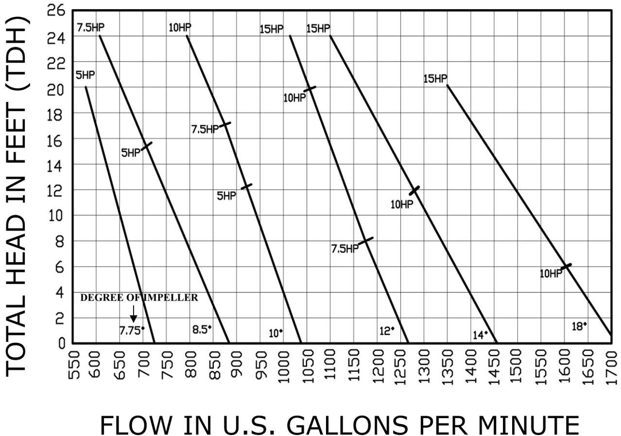
**PLOT YOUR POINT:** Follow the flow in U.S. gallons per minute required horizontally on the chart to your GPM flow required; then follow up to your total head in feet required.
